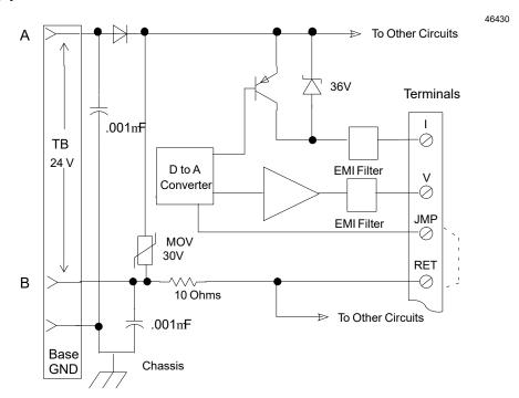
Each circuit provides simultaneous voltage and current outputs from the digital to analog converter. All circuits share a common loop supply and return.
