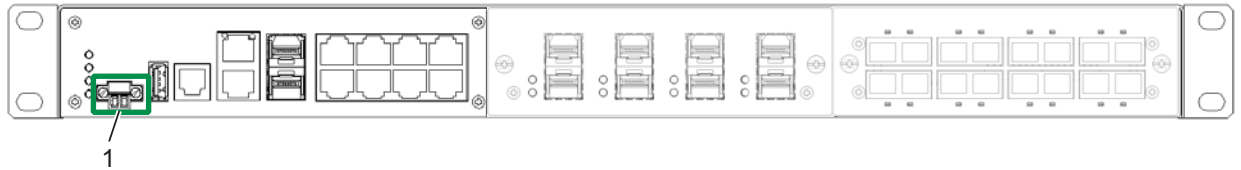
Figure 14: MACH102 device, front view 1 - Signal contact
