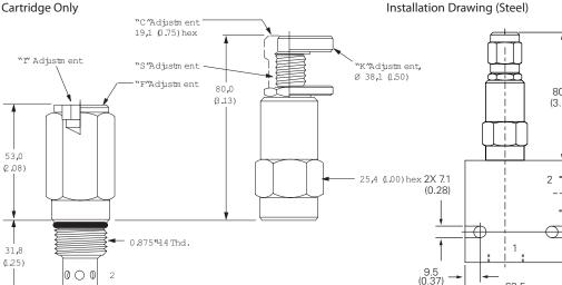
A - 47-54 Nm (35-40 ft. lbs) S - 68-75 Nm (50-55 ft. lbs) Installation Drawing (Steel)
